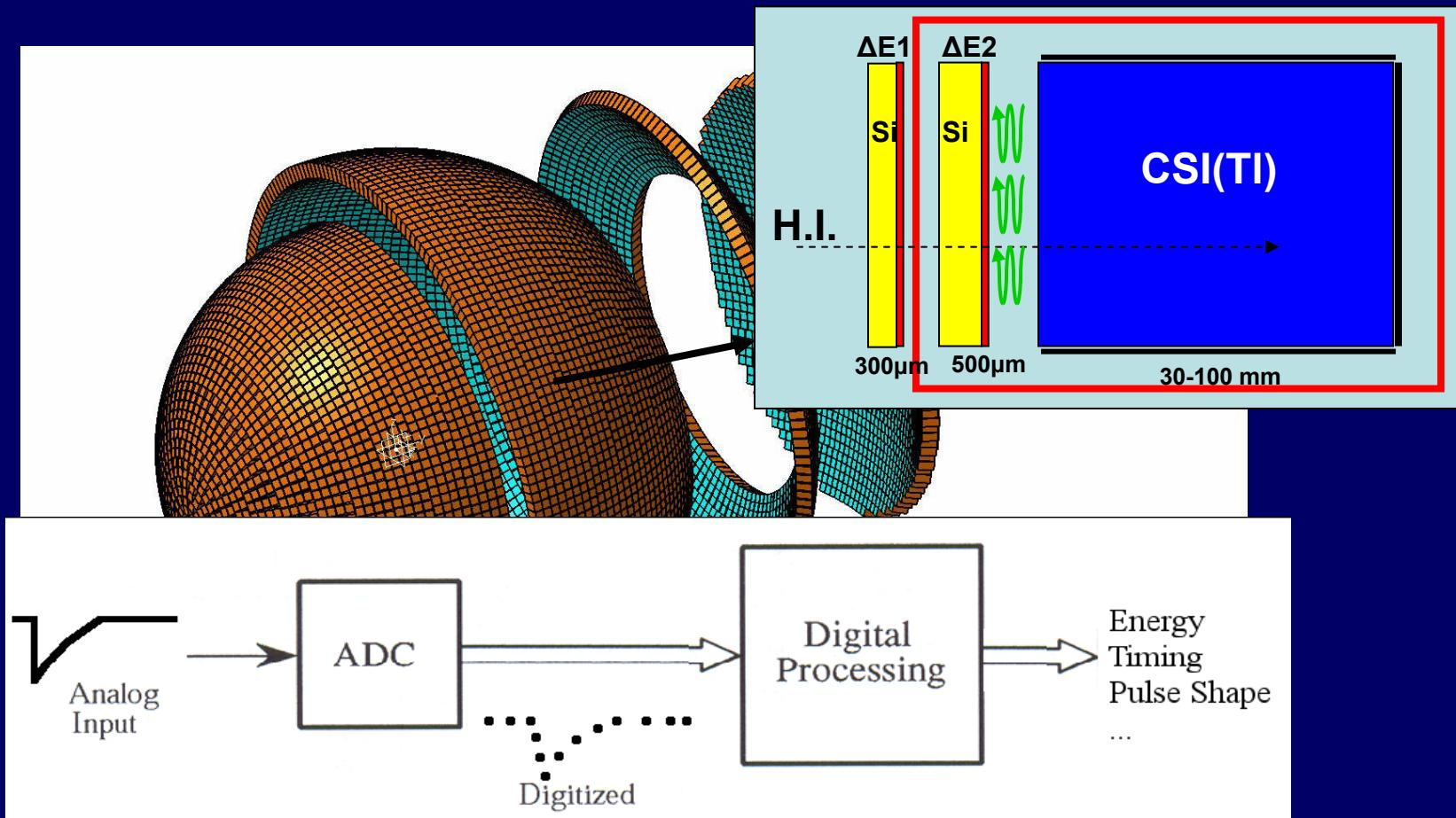
**Identify ions stopped in one silicon detector
