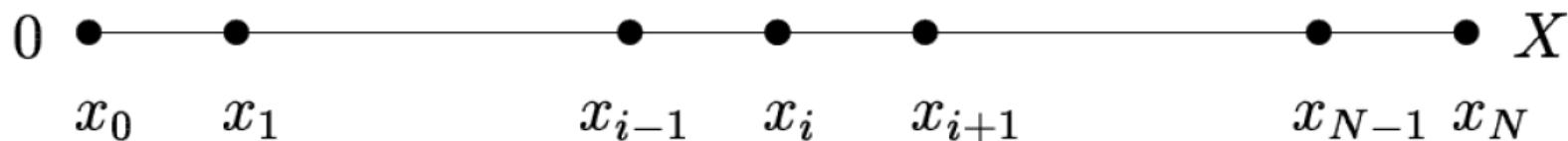
$$\left( \frac{\partial u}{\partial x} \right)_i = \lim_{\Delta x \rightarrow 0} \frac{u(x_{i+1}) - u(x_i)}{\Delta x} = \lim_{\Delta x \rightarrow 0} \frac{u(x_i) - u(x_{i-1})}{\Delta x}$$
