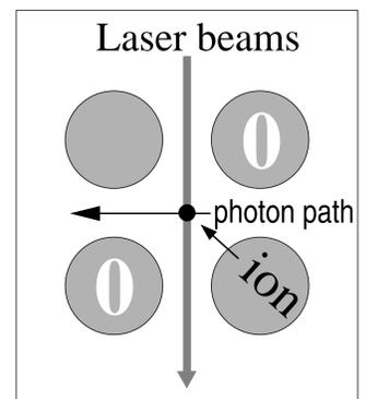
Laser beams carry out the STIRAP; Photon path is of the ring resonator.
