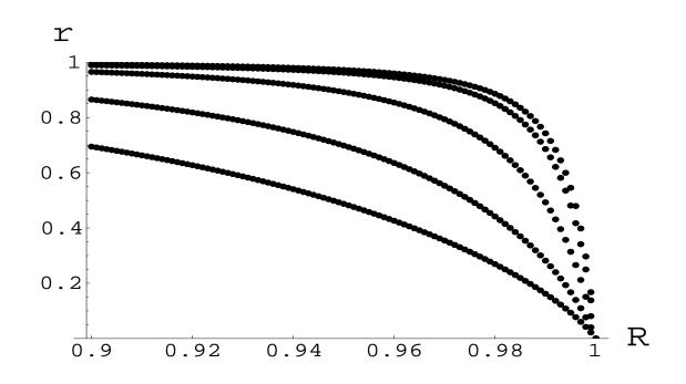
r as a function of  $\mathcal{T}/T$  for  $\rho=0.99$  and  $0.9 \leq R \leq 1$ :  $\mathcal{T}/T=500$  (top), 150, 50, 20, and 10 (bottom). The differences in the shapes stem from the amount of losses.
