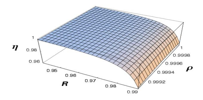
The efficiency of the suppression of the reflection into  $D_r$  when there is no object in the resonator;  $\rho$  is the measure of losses
