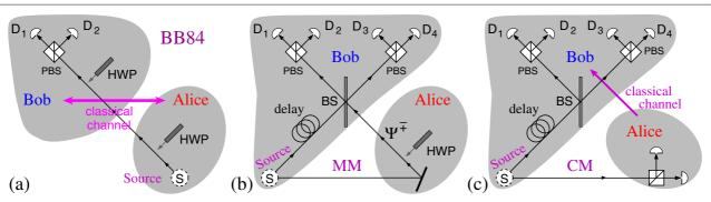
Fig. 1 Schematics of BB84 and ping-pong (pp) protocols. **a** BB84—classical and quantum channels are merged. **b** MM of the pp protocol—quantum channel. **c** CM of the pp protocol—classical channel
