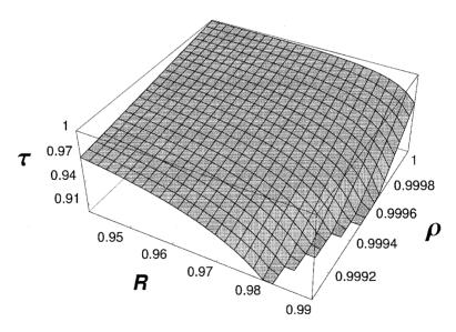
Fig. 6. The efficiency of the throughput into  $D_t$  when there is no object in the resonator as given by Eq. (9). R and  $\rho$  are defined as in Fig. 5.
