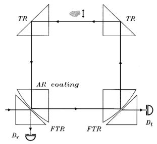
Fig. 4. Schematic of the proposed realistic interaction-free device. A single p-polarized photon tunnels (frustrated total reflection FTR) into the resonator. With a realistic efficiency exceeding 98% the beam makes several hundred loops guided by two total reflections TR and two FTR's to exit into  $D_t$ , when there is no object in the path. When there is an object in the resonator, the beam is reflected into  $D_t$ .
