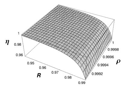
Fig. 5. The efficiency of the suppression of the reflection into  $D_r$  when there is no object in the resonator as given by Eq. (8). R is the frustrated total reflection at the two coupling output prisms and  $\rho$  is the measure of losses as defined for Eq. (1).
