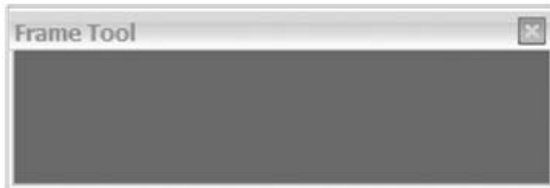
Figure 2.6 A toolbar frame, with a smaller title bar and no system menu
